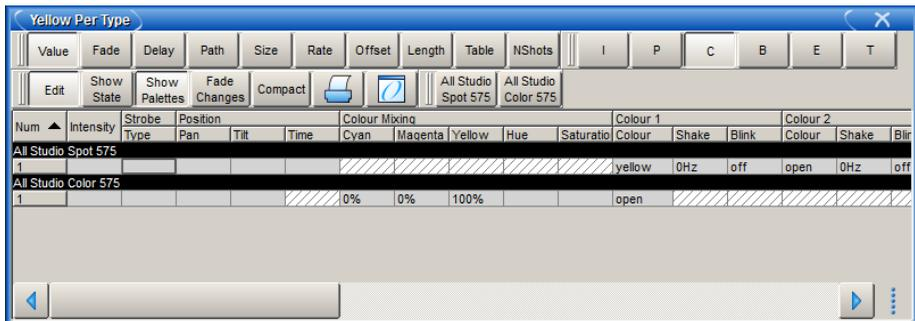
Figure 17.5. A Palette with Per Fixture Type Values
