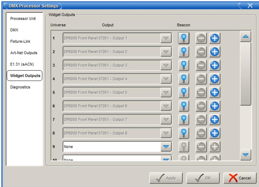
Figure 12.8. The Widget Outputs pane of the DMX Processor Settings window
