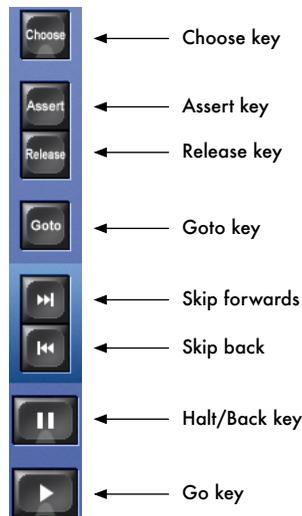
Figure 24.2. The Main Playback Controls
