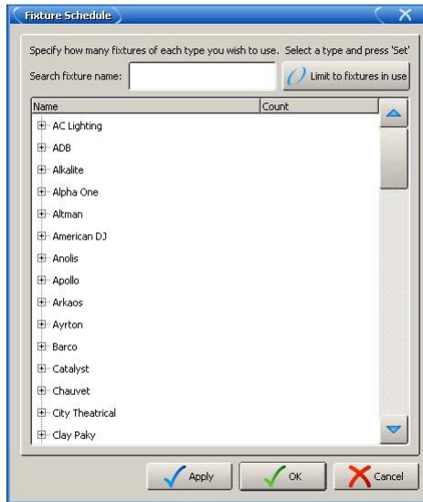
Use the trackball, mouse or cursor keys (below the trackball) to navigate the list of manufacturers. With the cursor keys, use up and down to scroll, and right and left to toggle open and closed each manufacturer's list.
