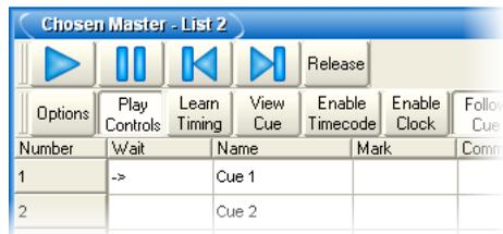
The controls are, from left to right, the Go, Halt/Back, Skip Back, Skip Forward, and Release buttons. These function in the same way as their front panel equivalents; see *The Main Controls* (p.267).
