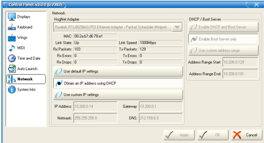
Figure 12.6. The Network pane of the Control Panel
