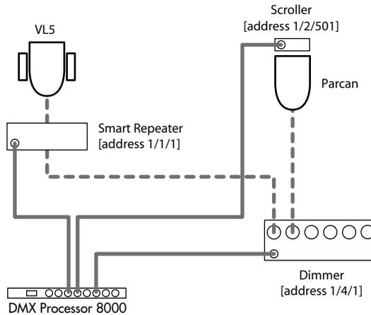
Figure 14.9. Examples of Fixtures requiring Multiple Patch Points
