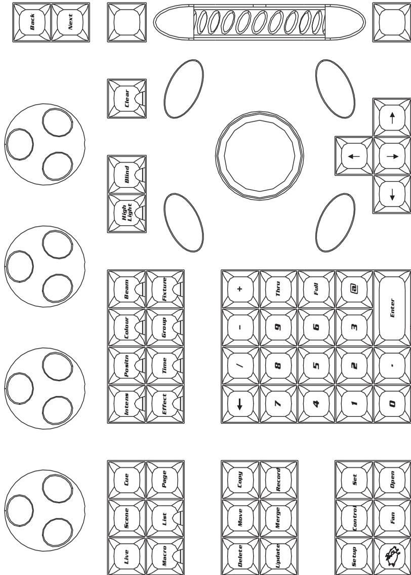
Figure 41.1. Programmer section of the front panel
