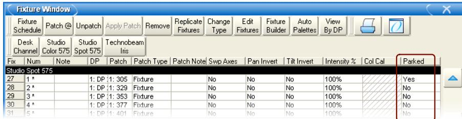
Figure 18.3. The Parked column of the Fixture window
