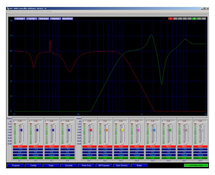
The M Series Processor is shipped with a special PC Graphic User Interface (GUI) application - XLink. XLink gives the user an option to control the M Series Processor from a remote PC via the RS232 serial communication link. The GUI application makes it much easier to control and monitor the device, allowing the user to get the whole picture on one screen. Programs can be recalled and stored from/to PC's hard drive, thus expanding the storage to become virtually limitless.
