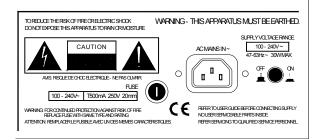
Refer to the **SAFETY WARNING** on page 5 of this Guide. Check that the correct mains lead with moulded plug has been supplied with your console. Read and understand the warnings and instructions printed on the rear panel and reproduced here. The power supply accommodates mains voltages within the range 100-240V without changing any fuses or settings.
