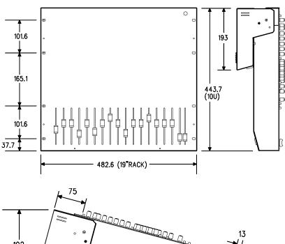
Mount the console in the rack using 4x M6 bolts each side for maximum strength. We recommend you fit the bolts with plastic cup washers to protect the panel, and they look good... These should be available from the supplier of the rack unit or a good hardware store.
